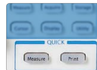
Auto Measure Button To turn on selected general measurements directly
