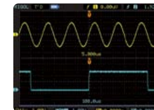
Alternate Trigger Provides a true dual timebase display
