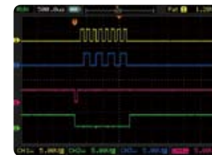
Pattern Trigger Triggers on any combination of events across all 4 analog channels
