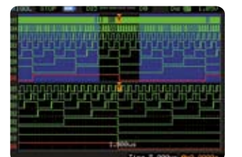
Duration Trigger A combination of Pattern Trigger and Pulse Width Trigger capabilities make isolation of events easy
